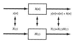
Fig. 4-3 Impulse response and system function.
