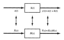
Fig. 3-7 Impulse response and system function.
