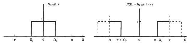
Fig. 6-22 Transformation of a low-pass filter to a high-pass filter.
