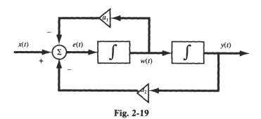
Let e(t) and w(t) be the input and the output of the first integrator in Fig. 2-19, respectively. Using Eq. (2.95), the input to the first integrator is given by
