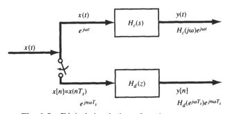
Fig. 6-5 Digital simulation of analog systems.
