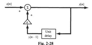
In Fig. 2-28 the output of the unit delay element is y(n-1). Thus, from Fig. 2-28 we see that
