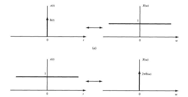
Fig. 5-20 (a) Unit impulse and its Fourier transform; (b) constant (dc) signal and its Fourier transform.
