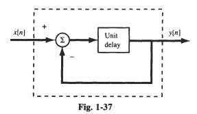
From Fig. 1-37 the input to the unit delay element is x[n] - y[n]. Thus, the output y[n] of the unit delay element is [Eq. (1.111)]
