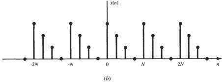
Fig. 1-3 Examples of periodic signals.
