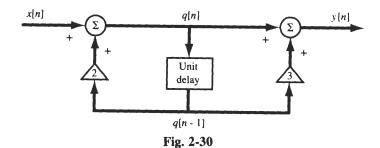
Let the input to the unit delay element be q[n]. Then from Fig. 2-30 we see that
