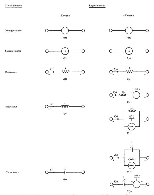
Fig. 3-10 Representation of Laplace transform circuit-element models.
