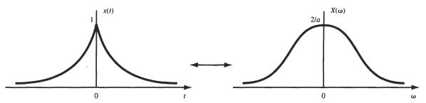
Fig. 5-18  $e^{-|a|t}$  and its Fourier transform.
