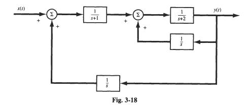
**3.55.** Determine the overall system function H(s) for the system shown in Fig. 3-18.
