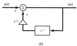
Fig. 6-28 Simulation of an RC filter by the impulse invariance method.
