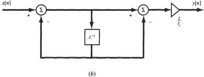
Fig. 6-30 Simulation of a differentiator.
