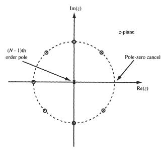
Fig. 4-4 Pole-zero plot with N = 8.
