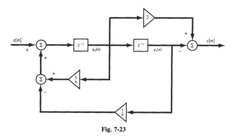
**7.56.** Consider the discrete-time LTI system shown in Fig. 7-24. Find the state space representation of the system with the state variables  $q_1[n]$  and  $q_2[n]$  as shown.
