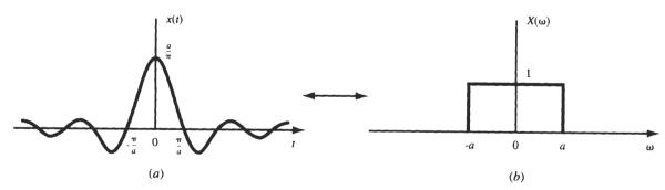
Fig. 5-17  $\sin at/\pi t$  and its Fourier transform.
