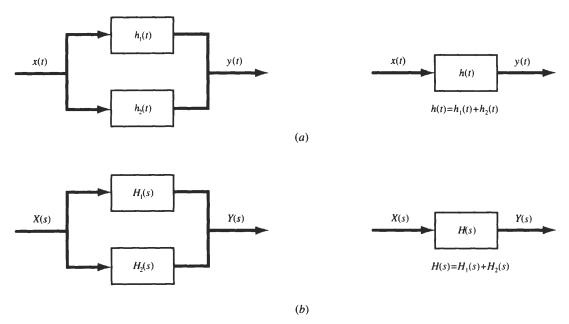
Fig. 3-9 Two systems in parallel. (a) Time-domain representation; (b) s-domain representation.
