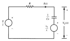
Fig. 3-15 Transform circuit.
