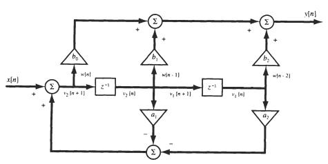
Fig. 7-9 Canonical simulation of the second form.
