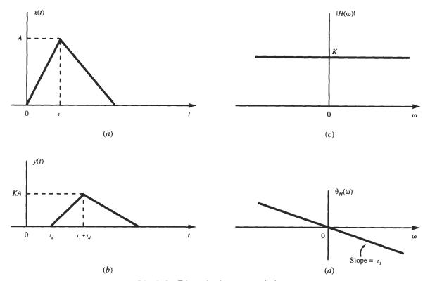
Fig. 5-4 Distortionless transmission.
