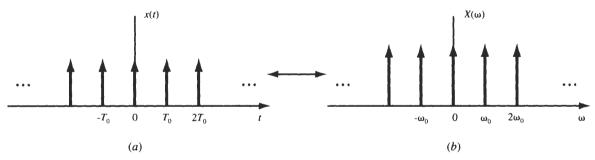
Fig. 5-22 Unit impulse train and its Fourier transform.
