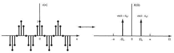
Fig. 6-15 A cosine sequence and its Fourier transform.
