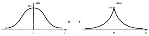
Fig. 5-19  $1/(a^2 + t^2)$  and its Fourier transform.
