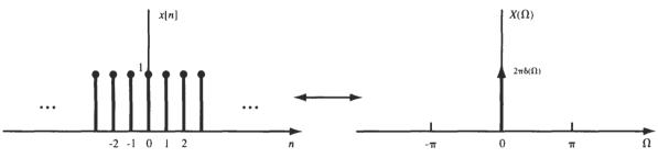
Fig. 6-14 A constant sequence and its Fourier transform.
