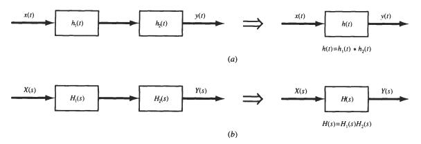
Fig. 3-8 Two systems in cascade. (a) Time-domain representation; (b) s-domain representation.
