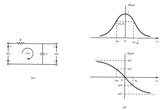
Fig. 5-6 RC filter and its frequency response.
